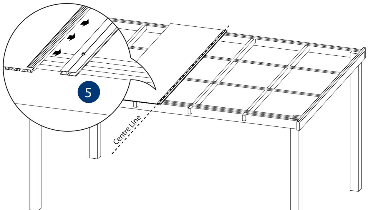
6. Apply Rubber Gasket and install the Second H profile aligning the end of each H profile
