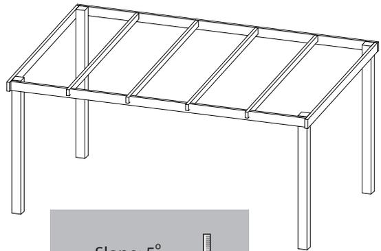
Make sure there is adequate fall of minimum 5 degrees (87mm per 1000mm). A good fall will aid in keeping the sheets clean.
