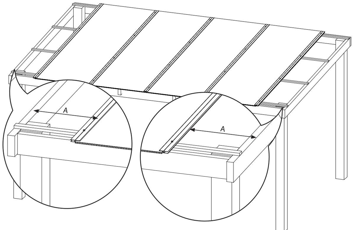
8. Cut the width necessary for both edge sheets.
