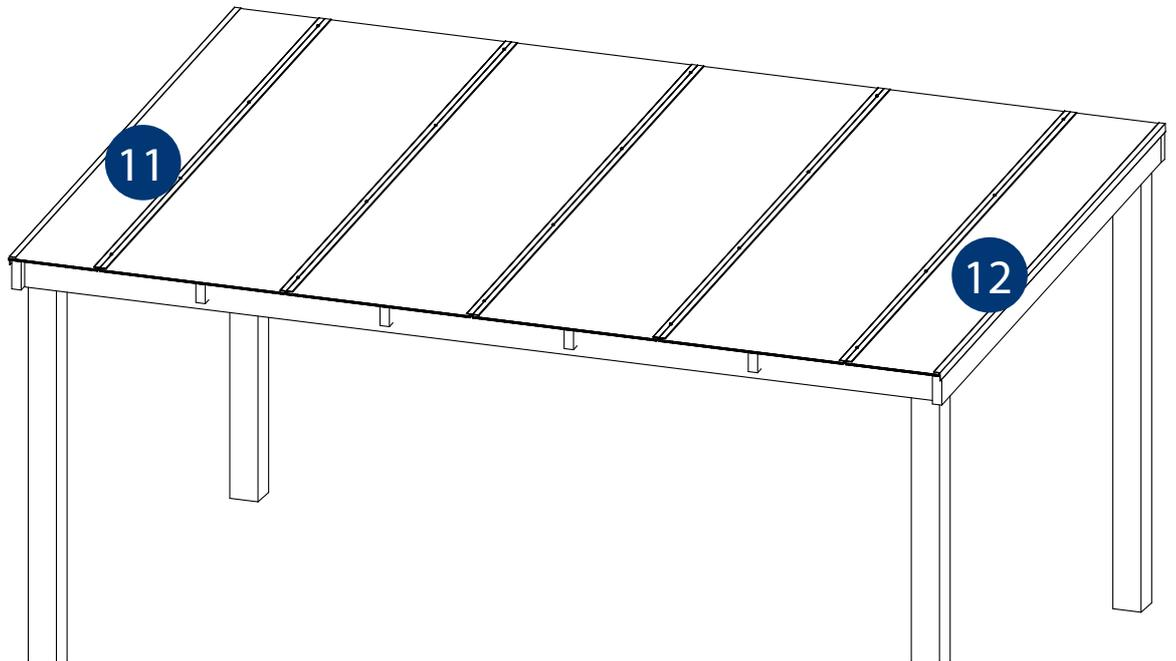
13. Align end edge of Sheet End Cap to outside edge of H Joiner or F Section. Tap & fit Sheet End Cap along top & bottom edge of sheeting to ensure a neat fit to H Joiner.
