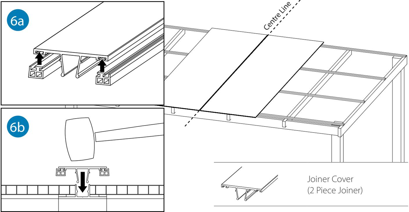
**7.** Install all SUNLITE sheets as shown in steps 1-6. Measure the uncovered area's width on both sides (A).
