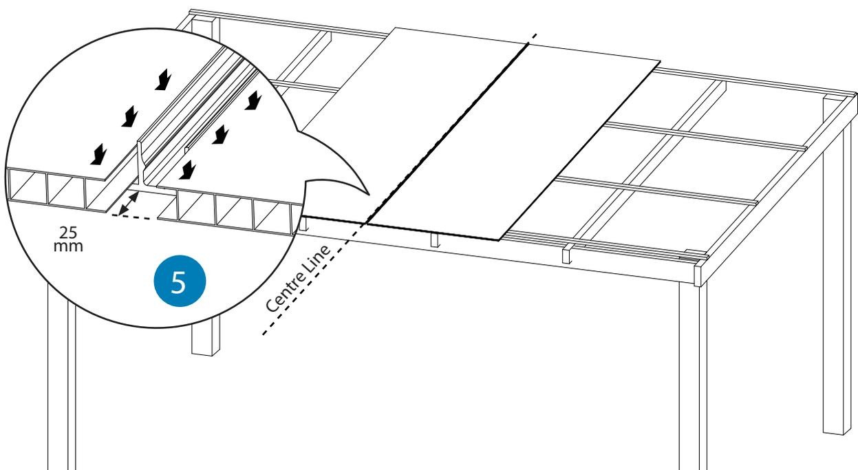
**6.** Cut to size and fix Captive Wedge with edge lip to outside edge of joiner Cover face. Make sure the cover profile and the captive wedge are aligned. Position the first Joiner Cover aligned with the first Joiner Base and secure the two profiles by using rubber mallet.
