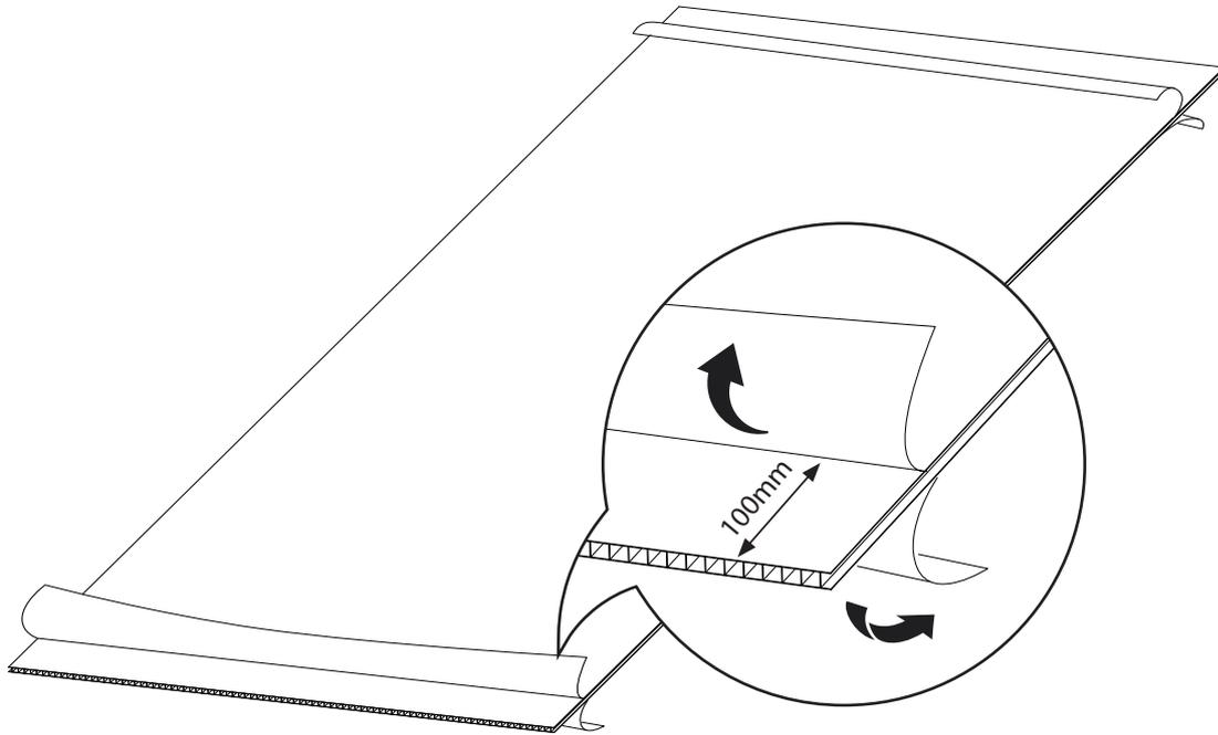
Apply the Blocking tape to the top end of the sheet, and carefully fold the protruding sides over both sheet faces to cover the internal channels.
