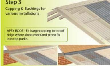
AGAINST A WALL/FASCIA - Fit barge capping to edge of sheet and apron fashing at the wall or fascia. Secure using recommended fixing screws.
